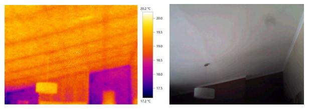
**21.** Thermography of kitchen A/C: seems dry enough underneath. Possible slight damp patch low down / at the noggings. Often an occasional overflow in humid weather, and/or the condensate pipe is leaking / blocked.
